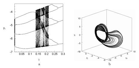
**Fig. 2.** Phase-parametric characteristic (a) and phase portrait of the chaotic attractor (b)
